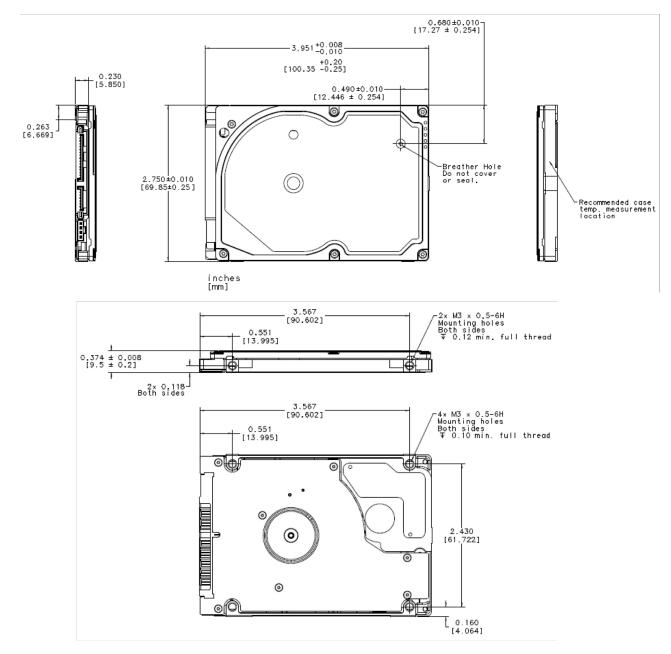
Figure 3. Mounting dimensions-top, side and end view
